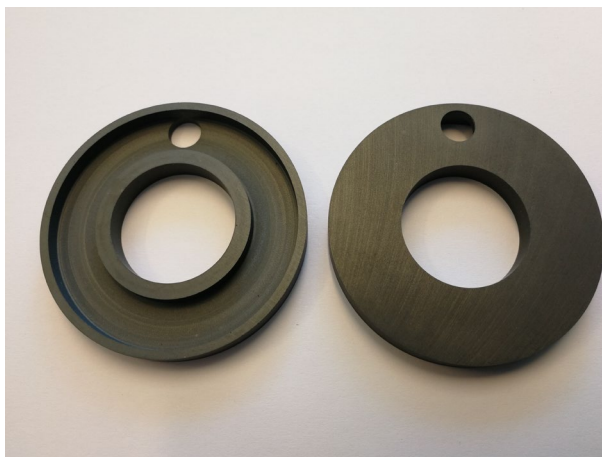
(a) Ferrite pot cores.
